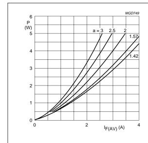
Fig.4 Maximum steady state power dissipation (forward plus leakage current losses, excluding switching losses) as a function of average forward current.
