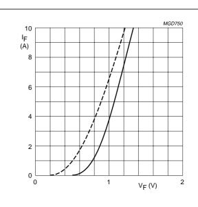
Dotted line:  $T_j = 175 \,^{\circ}\text{C}$ . Solid line:  $T_j = 25 \,^{\circ}\text{C}$ .
